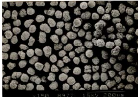
Fig. 1. Image of the crystalline aggregates of particle size 36-40 \mu\text{m} used for the modeling process. SEM.
