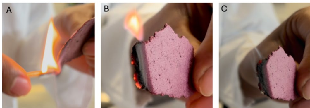
Fig. 6. Interaction of the generated material with a lit match (A), the fire interacts with the material (B), and after 10 s, it goes out (C).
